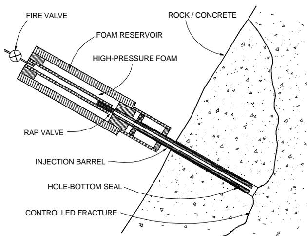
Figure 1. Basic hardware and geometry for controlled foam injection (CFI) fracture of rock.
