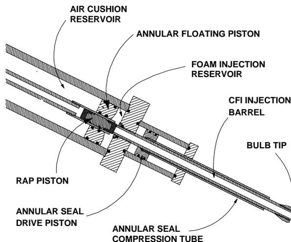
Figure 2. Details of reverse acting piston (RAP) valve and of annular floating piston in CFI breaker.
