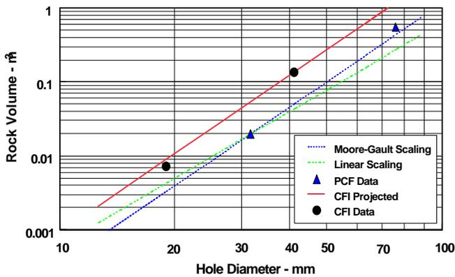
Figure 4. Log-log graph showing nonlinear scaling of CFI and PCF rock breakage.
