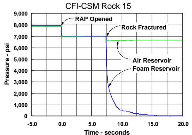
Figure 3. Pressure records from a CFI rock breaking test showing delayed rock fracturing.
