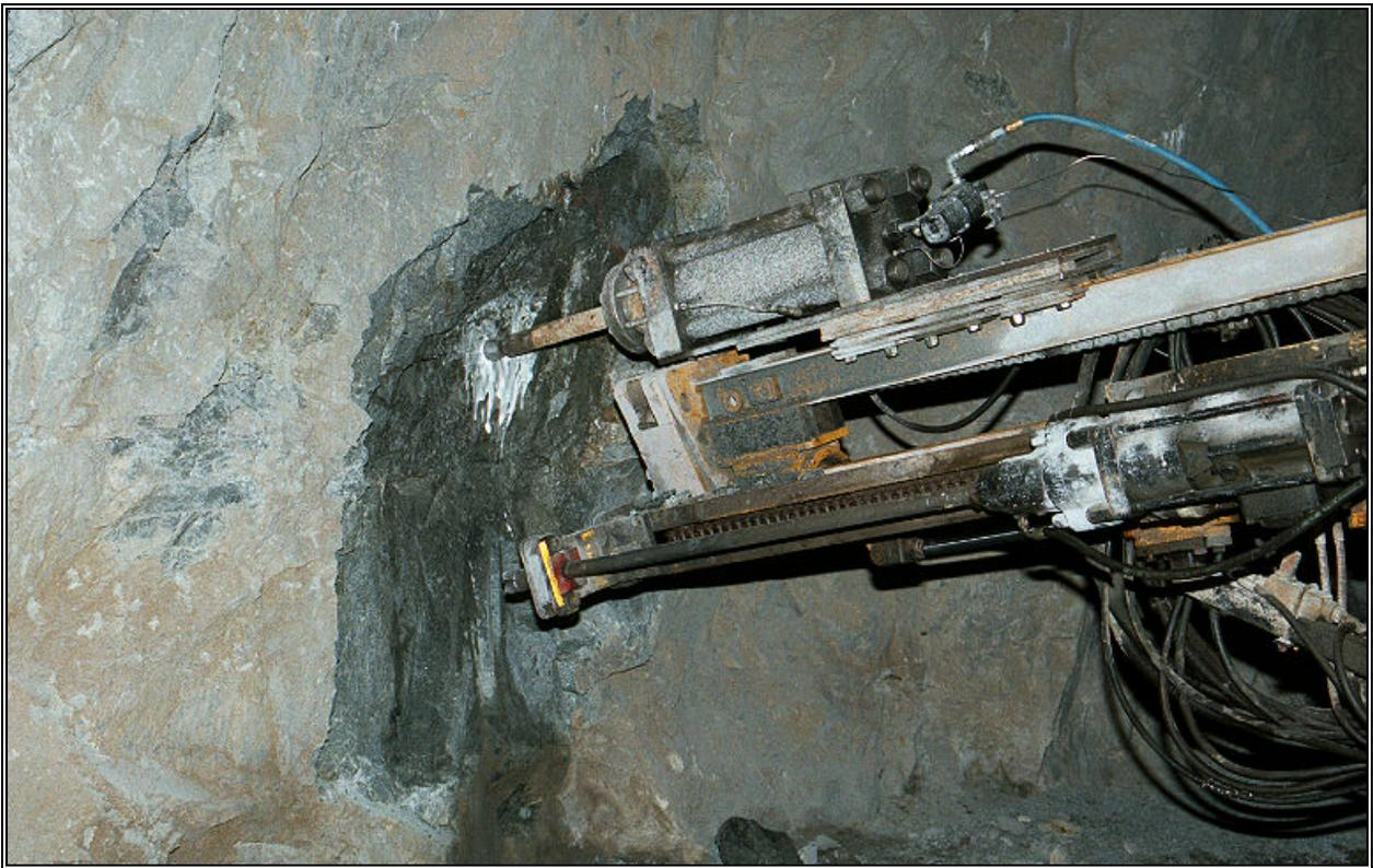
**Figure 5. Photograph of CFI breakage from the first test conducted at the second Fecunis Adit location.**
