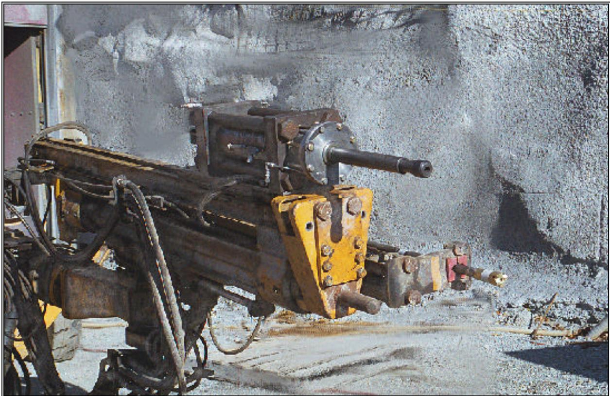
**Figure 3. Photograph of 51 mm CFI breaker mounted with a drill on the indexing boom of the MacLean 829 carrier.**
