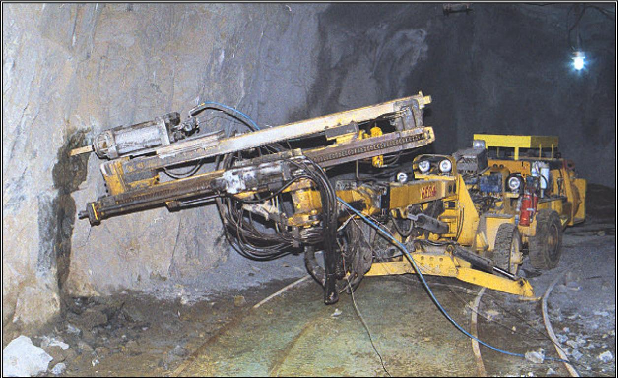
**Figure 4. Photograph of the MacLean 829 positioned for the first CFI break at the second Fecunis Adit location.**
