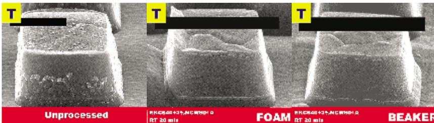
**SEMs compare the unprocessed wafer (left) with cleaning results using foam (middle) or liquid (right) medium, demonstrating equivalent cleaning results. (Source: Aquafoam).**
