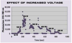
Results show that increasing the power to the transducers beyond a saturation level has a deleterious effect on the amount of cavitation generated, as well as on cleaning efficiency. (Source: SEZ America)
