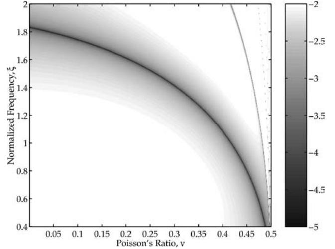
FIG. 3. Contour plot of the logarithm of the characteristic function,  $\log_{10}(|C|)$ , for the  $n=2$  spheroidal mode of an elastic sphere. Dark contours corresponding to low values of  $C$  represent the natural frequencies of the sphere.
