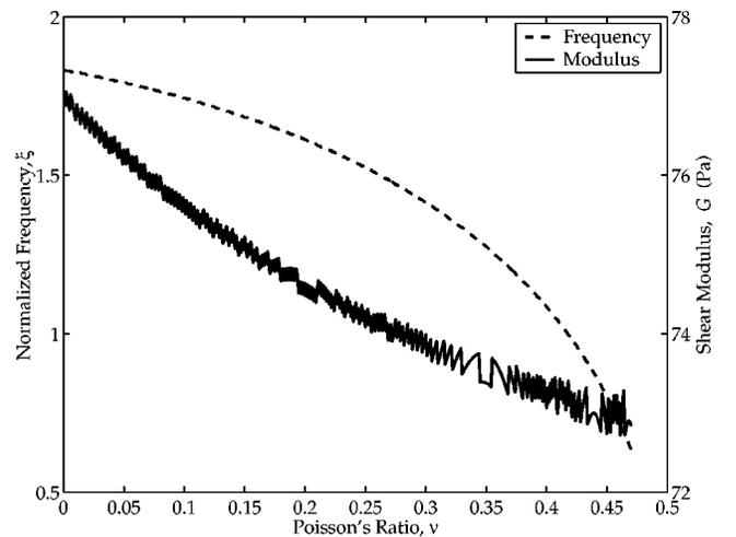
FIG. 4. Plot of the  $n=2$  fundamental spheroidal frequency of an elastic sphere, obtained by extracting the lower contour of Fig. 3. Plotted against the right-hand ordinate is the corresponding shear modulus of a foam drop that would resonate at 63 Hz.
