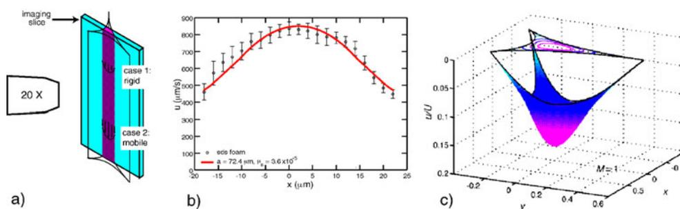
**Figure 2.** (a) The experimental configuration for confocal imaging of the flow in a single Plateau border. (b) The velocity profile across a Plateau border during drainage where the symbols show measurements and the solid curve is based on a model of flow along the channel with transverse shearing of a surfactant film. (c) A three-dimensional view of the numerically computed velocity profile when the interfaces exhibit flow due to interfacial mobility (Koehler *et al* 2002).
