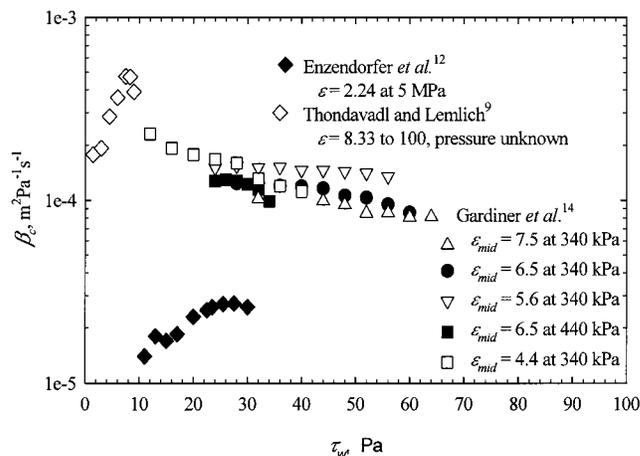
**Figure 2.** Collation of slip coefficients determined for three separate experimental studies. Both Wenzel et al.<sup>8</sup> and Enzendorfer et al.<sup>12</sup> observe a slip coefficient that increases with wall stress up to a limiting stress. At the high shear rates of Gardiner et al.<sup>14</sup> the slip coefficient was observed to decrease with wall stress.
