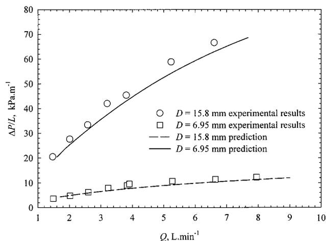
**Figure 7.** Comparison of the pressure loss predictions of eq 20 with Gardiner et al.'s<sup>14</sup>  $\epsilon_{\text{mid}} = 6.5$  flow data for two pipe diameters and gauge pressure of 340 kPa. The slip velocity was determined from the  $\epsilon$ -dependent scaling curve found in Figure 3.
