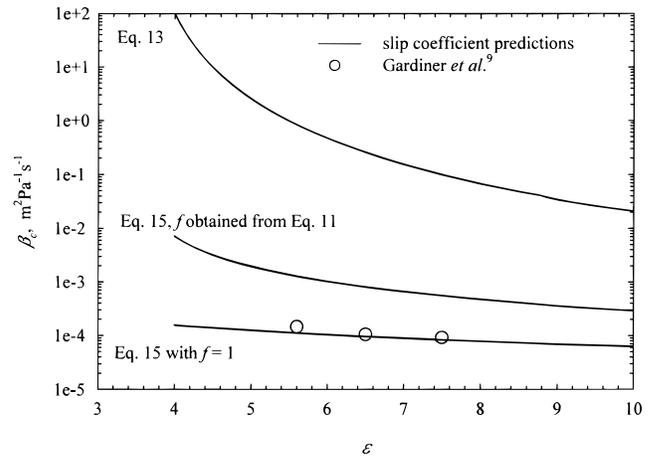
**Figure 6.** As the high shear rates of Gardiner et al.<sup>14</sup> limit the rate of availability of liquid to form the slip layer, a second model, eq 15, is considered to account for restrictions on slip layer formation:  $\sigma = 0.025$  N/m;  $\langle R \rangle = 80$   $\mu\text{m}$ ;  $D = 0.01$  m;  $\tau_w = 50$  Pa;  $\mu = 0.001$  Pa s;  $\Delta R = \langle R \rangle$ .
