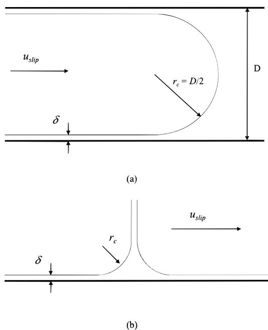
**Figure 4.** Illustration of (a) Bretherton's<sup>24</sup> analysis of the flow of a long bubble down a tube and (b) the motion of a single Plateau border near a wall.
