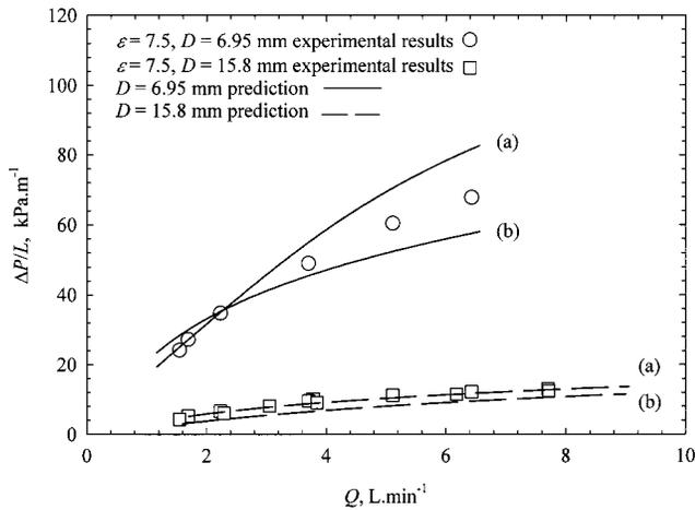
**Figure 8.** Comparison of the pressure loss predictions of eq 20 with Gardiner et al.'s<sup>14</sup>  $\epsilon_{\text{mid}} = 7.5$  flow data for two pipe diameters and gauge pressure of 340 kPa. The slip velocity was determined by (a) the  $\epsilon$ -dependent scaling curve found in Figure 3, and (b) the predictions of eq 15 with  $f = 1$ .
