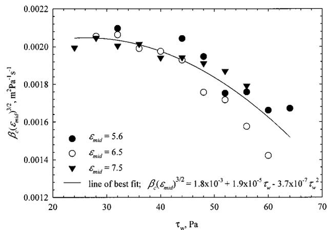
**Figure 3.** When Gardiner et al.'s<sup>14</sup> constant pressure slip coefficient results are scaled by  $(\epsilon_{\text{mid}})^{3/2}$ , the data from three expansions can be fitted to a single curve.<sup>19</sup>
