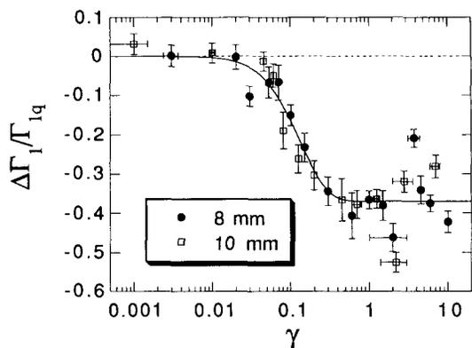
FIG. 3. Fractional change in the cumulant immediately following a shear step strain of size  $\gamma$ ; the plate separations are as labeled, and the solid curve is a guide to the eye. Results are for roughened plates, and uncertainty in strain due to both uncertainty in total plate motion and wall slip is denoted by horizontal error bars.
