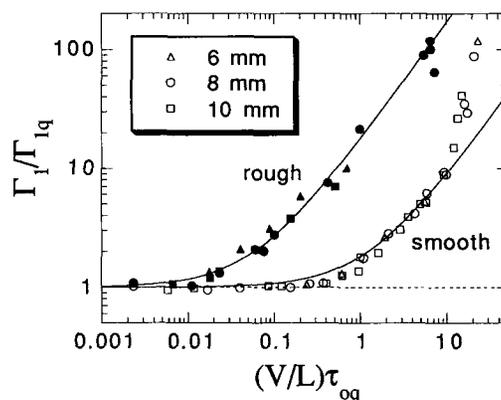
FIG. 4. Ratio of the first cumulant for a foam under shear to that of a quiescent sample of the same thickness,  $L$ , vs Deborah number;  $V$  is the velocity difference imposed between top and bottom plates and  $\tau_{0q} = 20$  s. Open (solid) symbols are for smooth (roughened) plates. Solid curves are fits, indicating that coarsening-induced rearrangements dominate at small  $(V/L)\tau_{0q}$  while shear-induced rearrangements increase proportional to the strain rate.
