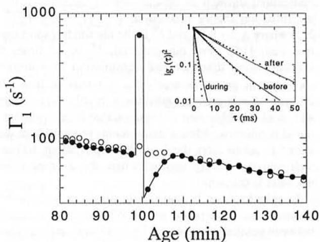
FIG. 1. First cumulant vs foam age for a quiescent sample (open circles) and one that is sheared from 98 to 100 min (solid circles connected by lines); the plate velocity for the latter is  $V = 4 \text{ mm/s}$ , and the plate separation is  $L = 8 \text{ mm}$ . The inset shows raw autocorrelation data (symbols) and fits (curves) before, during, and after application of shear.
